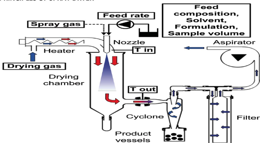
Figure 1: Process diagram of the Mini Spray Dryer B-190, B-191 and B-290 models with process parameters.
