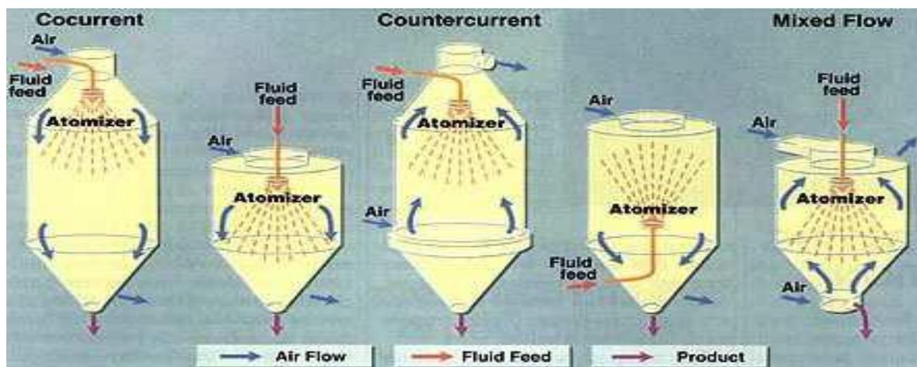
**Fig.3:** The atomized droplets that are formed from the atomizing device established by the atomizer
